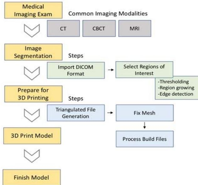
Overview of the process of using medical imaging data to produce a 3D-printed anatomical model, courtesy of Andy Christensen
