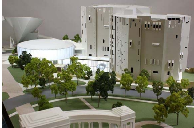
Art museum model containing parts made by binder jetting, vat photopolymerization, powder bed fusion, and laser cutting, courtesy of LGM
