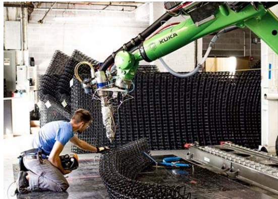
Robotic additive manufacturing at Branch Technology, courtesy of SHoP Architects
