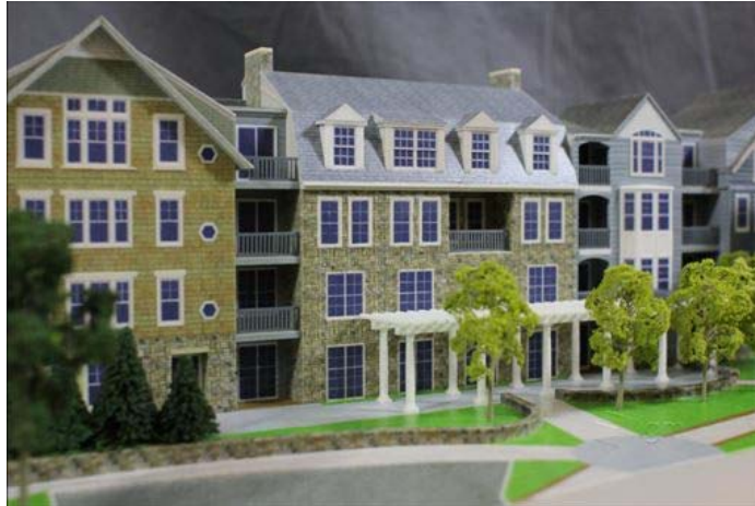
Color 3D-printed model of a multi-family residential project, printed on a ProJet 660 from 3D Systems, courtesy of LGM
