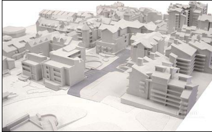
Large planning model at 25.4 mm = 4.9 m (1 inch = 16 ft) scale, printed on ProJet x60 from 3D Systems, courtesy of LGM
