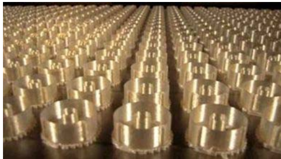
Build platform with 100 ULTEM 9085 toroid housings, courtesy of Stratasys
