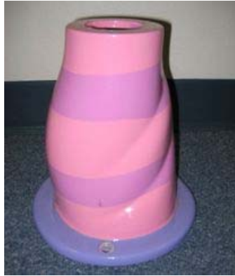
Pattern-based sand casting for an Orlando theme park ride part, courtesy of Mydea Technologies
