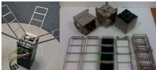
Assembled CubeSat satellite (left) and laser-sintered parts (right), courtesy of the RAMPART CubeSat team
