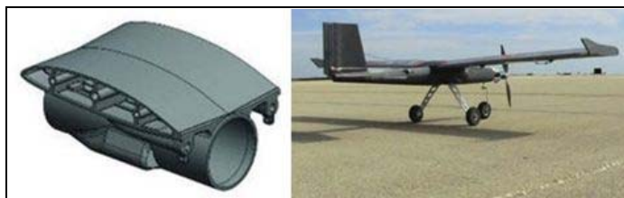
CAD image of fuselage-to-wing interface for UAV (left) and UAV on flight line (right), courtesy of Stratasys
