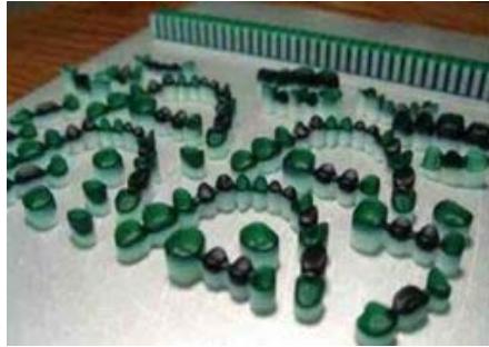
Build platform of waxups for copings, crowns, and bridges, courtesy of 3D Systems
