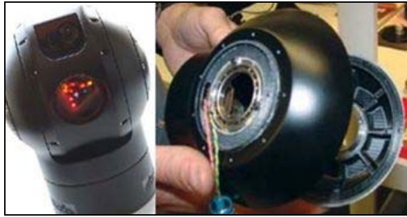
Gimbal eye for unmanned aerial vehicle (left) and FDM parts (right), courtesy of DST Control
