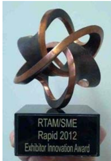
Innovation trophy designed by Bathsbeba Grossman, laser sintered at Harvest Technologies, and coated with copper, courtesy of Mcor
