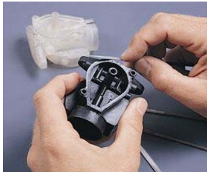
AM-produced master pattern (upper left) and molded urethane casting (center), courtesy of Met-L-Flo
