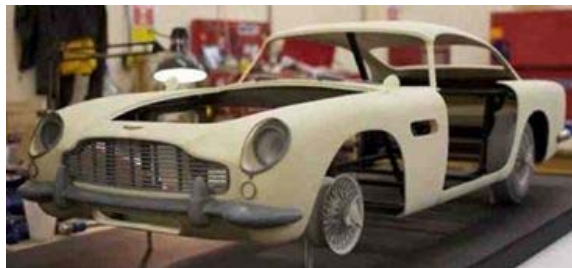
3D-printed Aston Martin DB5 replica, courtesy of Propshop Modelmakers Ltd. (now Voxeljet UK Ltd.)
