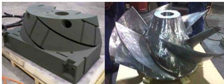
One half of split core (left) and finished impeller (right), courtesy of ExOne
