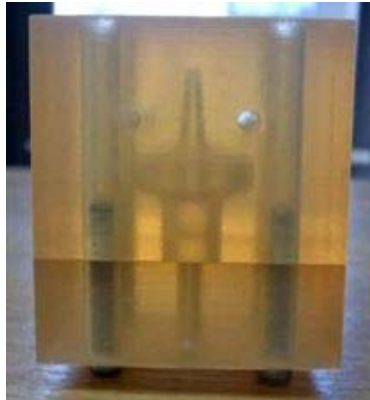
Three-piece stereolithography tool for rubber molding, courtesy of Met-L-Flo
