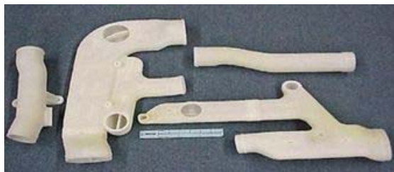
Environmental control system ducting, courtesy of Boeing
