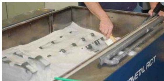
Technician cleans sand molds manufactured with an AM sand process, courtesy of Ford Motor Company
