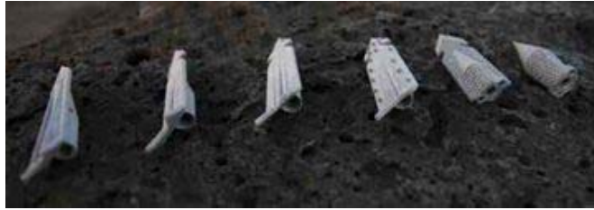
A lineup of fish tags, showing progression of the design from the earliest (left) to the latest prior to fitting with wires and electronics, courtesy of CSIRO
