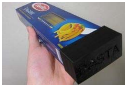
Pasta box end cap produced on a MakerBot machine, courtesy of Billy Zelsnack
