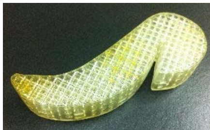
QuickCast stereolithography pattern used for metal investment casting, courtesy of Mydea Technologies
