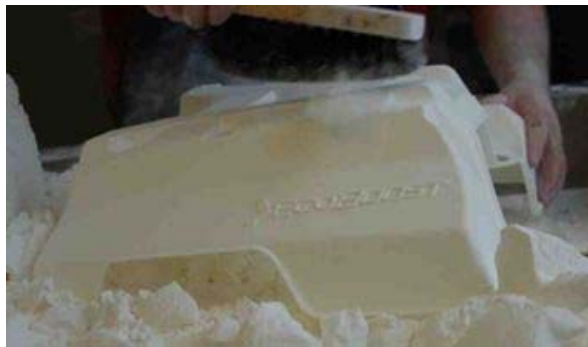
Technician brushes nylon powder residue from an EcoBoost engine prototype, courtesy of Ford Motor Company
