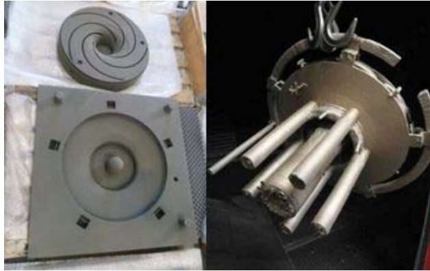
Sand mold and core (left) and unfinished casting (right), courtesy of Voxeljet
