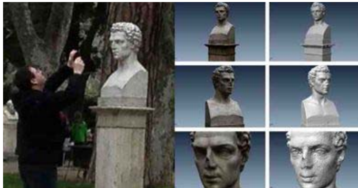
Low-cost digital camera used for 3D scanning a marble bust (left), and the scan data and conversion to a 3D model (right), courtesy of Direct Dimensions, Inc.
