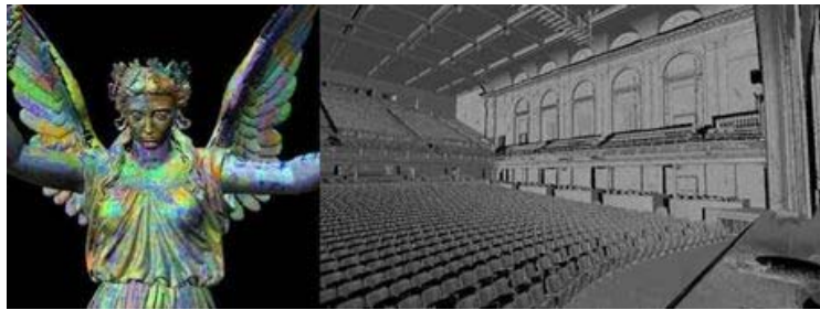
Most scanners capture dense data requiring sophisticated post-processing software, as shown in these scans of a sculpture and the interior of the Lyric Theatre, courtesy of Direct Dimensions, Inc.
