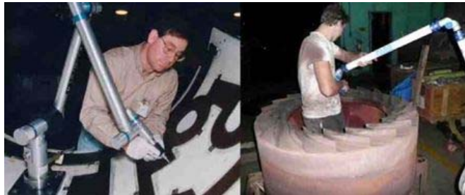
Two examples of portable articulated arm CMMs being used for 3D measurement in a manufacturing environment, courtesy of Direct Dimensions, Inc.
