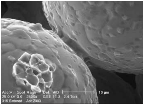
FIGURE 5 Electron micrograph showing a thermal bond produced through sintering to ensure predictable strength and dimensions. Source: Extrude Hone/ProMetal, 2003.
