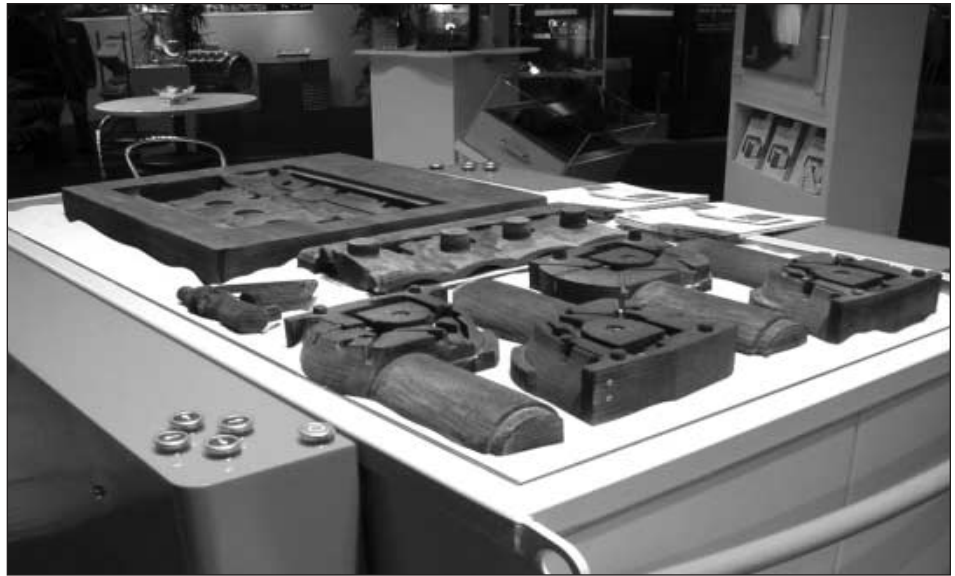
FIGURE 1 Molds for an engine set that can be produced in 36 hours with a build-box the size of a trunk. Source: Extrude Hone/ProMetal, 2003.
