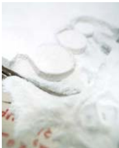
Breaking out: Pieces of replacement bone, complete with micropore structures, emerge from an ink-jet printing process.
