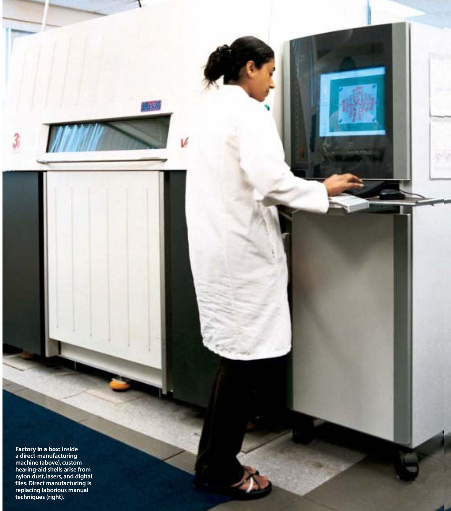
**Factory in a box:** Inside a direct-manufacturing machine (above), custom hearing-aid shells arise from nylon dust, lasers, and digital files. Direct manufacturing is replacing laborious manual techniques (right).
