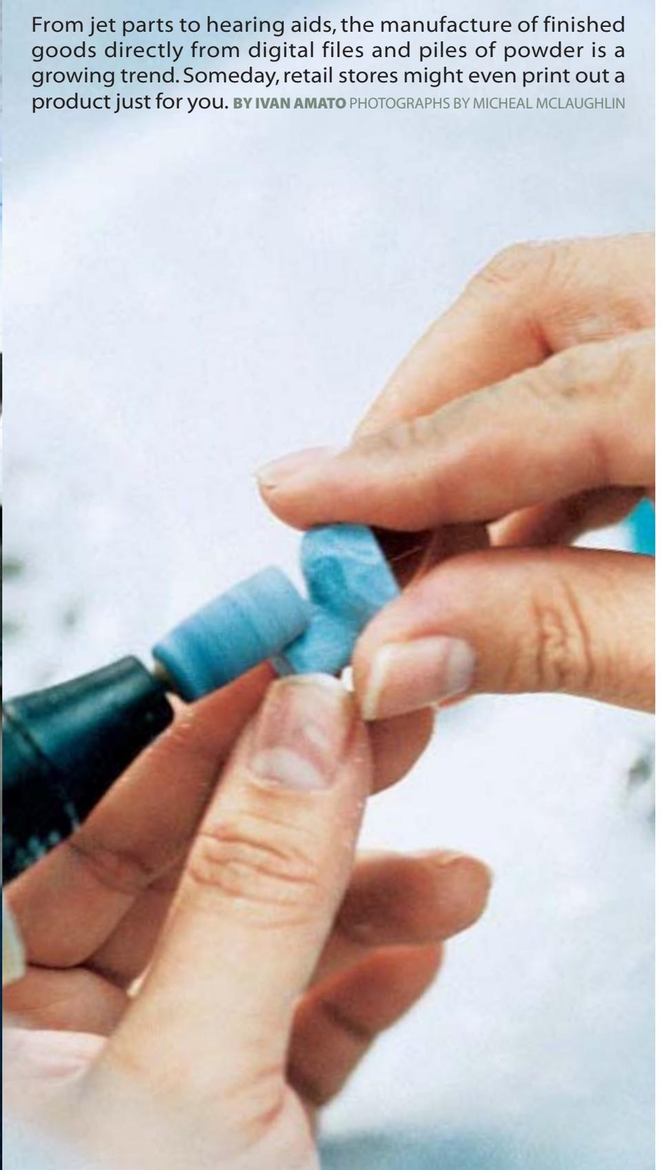
**A** boundary line of manufacturing history cuts across the factory floor of Siemens Hearing Instruments in Piscataway, NJ. On one side, skilled technicians use casting techniques, precision tools, and years of experience to craft the acrylic shells of hearing aids modeled from silicone impressions of actual ear canals.
