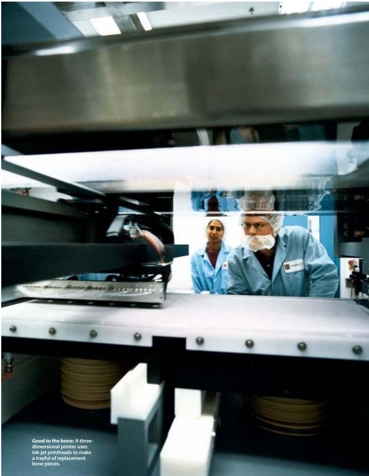
**Good to the bone:** A three-dimensional printer uses ink-jet printheads to make a trayful of replacement bone pieces.
